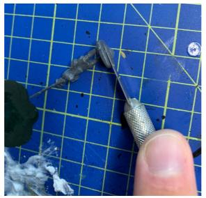
Here, I'm using a craft knife to slice away a lump of plastic from a base. You can also use a pocket knife blade or even a nail clippers for this. You won't need to use much force to slice through the plastic.
